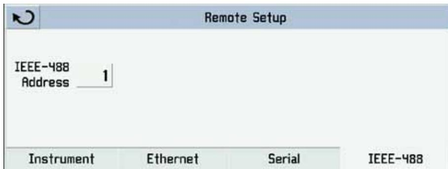
This screen is for setting the IEEE-488 address. Touch the numeric value box and a number entry keypad will appear for you to enter your new IEEE-488 address and then press [OK].
