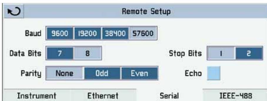
These parameters should be set to match your host computer. Default settings are: 57600 baud, 8 data bits, 1 stop bit, no parity, and no echo.
