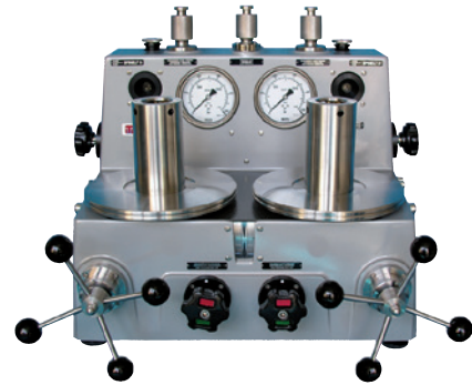
Primary-standard differential pressure balance, model CPB6000DP
