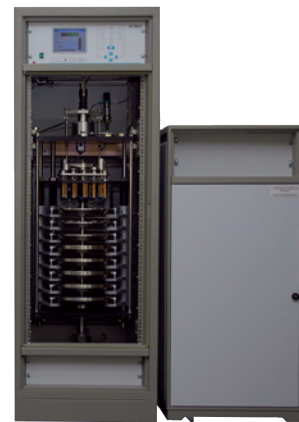
Automatic pressure balance, model CPB8000
